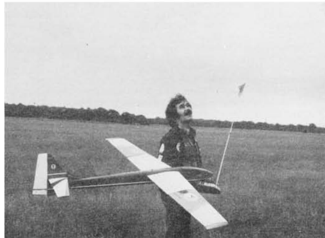
Wolfgang Schluter, LSF coordinator, Germany, and original "Inkognito." Fully aerobatic with rudder, elevator ailerons, spans 2050 mm (about 81 in.), weighs 1.6 kilograms (about 1.3 lbs.), modified Eppler 180.
