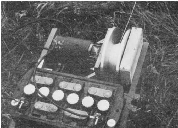
Winch powered by 12V Opel starter motor, used by sailplane group in Hannover, Germany. First attempt with such launching methods a breakthrough for fliers on continent. Impressive performance. Pruss pic.
