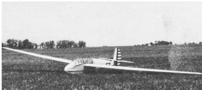
Jack Hiner's Schweizer TG-2 is 1/5 scale with 126-in. wing. Wing two-piece plug-in type. Red, yellow, white and blue coloring. Different!
