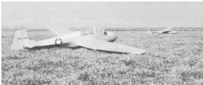
Mark Weber's Schweizer TG-3A, from plans by Jack Hiner, is 1/6 scale with scale surface areas—stab is 10%. the 3-1/2-lb. ship has coupled ailerons and rudder. In background, Hiner's KA-6. Jack Hiner photo.
